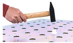
To recreate the Vario-Bench's incremental 1° hole pattern, mark the holes using the supplied marking kit...
