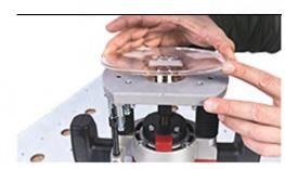
Attach the routing kit supplied with the product to your router to enable precise positioning of the holes.
