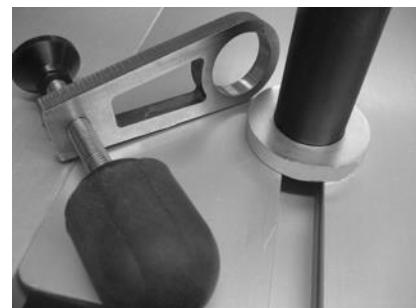
The distance between the T-slot and the saw blade is determined by the swivel arm length.
