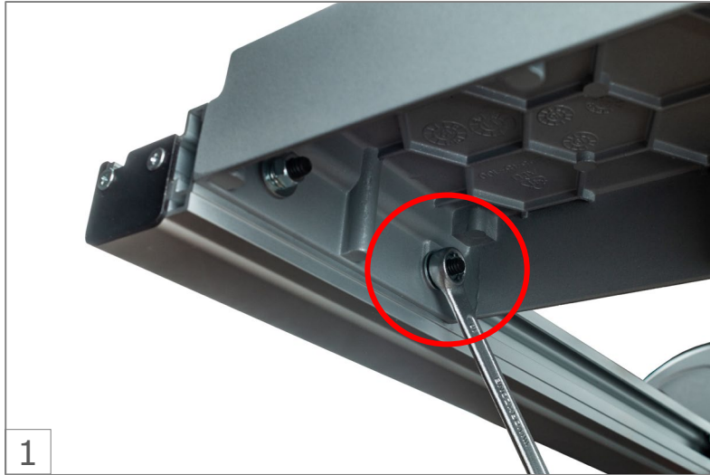
1 Loosen all 4 screws at the end of the table extension.
