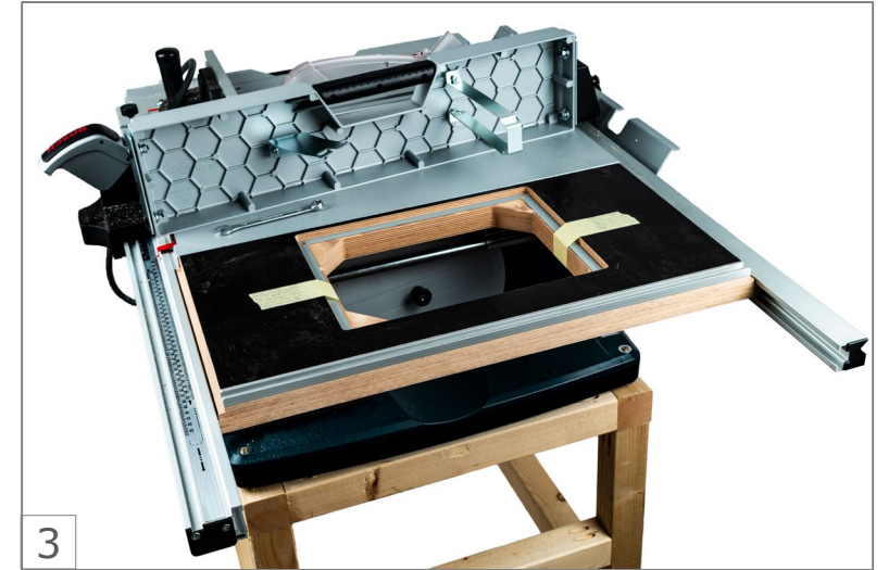
3 Push the router table plate FTP-GTS10 between the grooves as far as possible.
