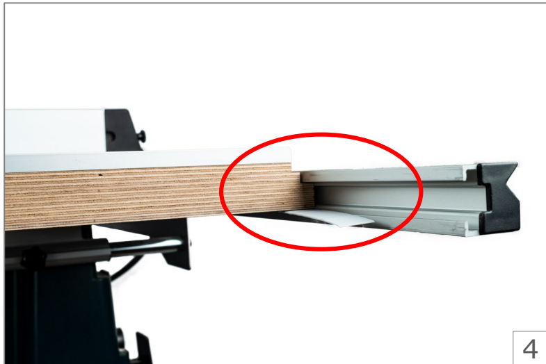
4 If necessary, use the shims to compensate for any height differences (supplied).
